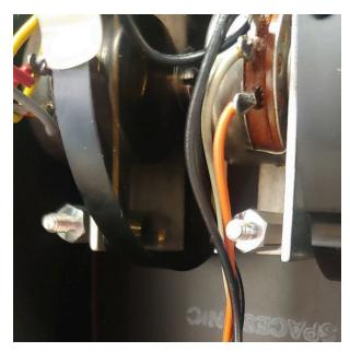
**3. MOUNTING.** Two standoffs must be installed to mount the "Bender Perfecter" board.
