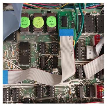
Insert the Memory Liberator board into the socket where U5 originally was. Insert the free end of the ribbon cable connected to the mod board into the socket where U11 was. The U22 socket will be left empty.
