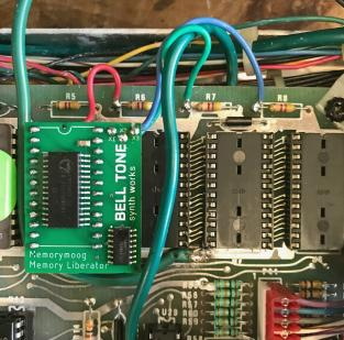
Insert the Memory Liberator board in the socket where the leftmost of the RAM chip (U5) used to be.
