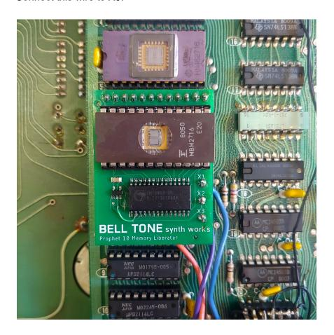
Insert the Memory Liberator board into the socket that previously held the EPROM that you removed, as shown, with the half-circle divot on the silkscreen facing to the left as seen in the photo.
