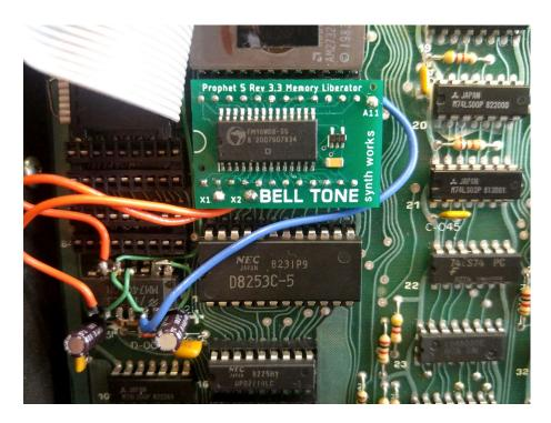
Carefully tack-solder two new wires to the ugly mod IC (known as U387) at pins 6 and pin 8 (orange wires in photo). Be careful not to disturb the connections that have already been made on U387. Solder one of these wires to the "X1" pad on the Memory Liberator board and the other to "X2." It doesn't matter which is which.
